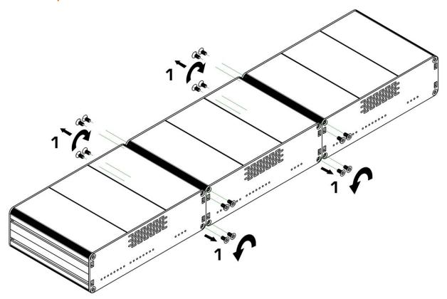
4.2 Step 2 to 5 : Screw 4x fasteners and 2x small ears as below
