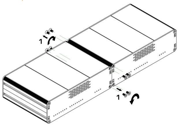
3.2 Step 2 to 5: Screw 2 fasteners + 1 long ear + 1 small ear as below
