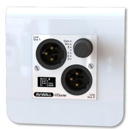
The AV-WALL-DT4o-B is a single-gang wall mounted Dante and Bluetooth output audio interface. The compact design provides a flexible and easy to use installation solution. It is PoE enabled so you only require one Cat5e/6 cable to connect the power, control and transmission.
