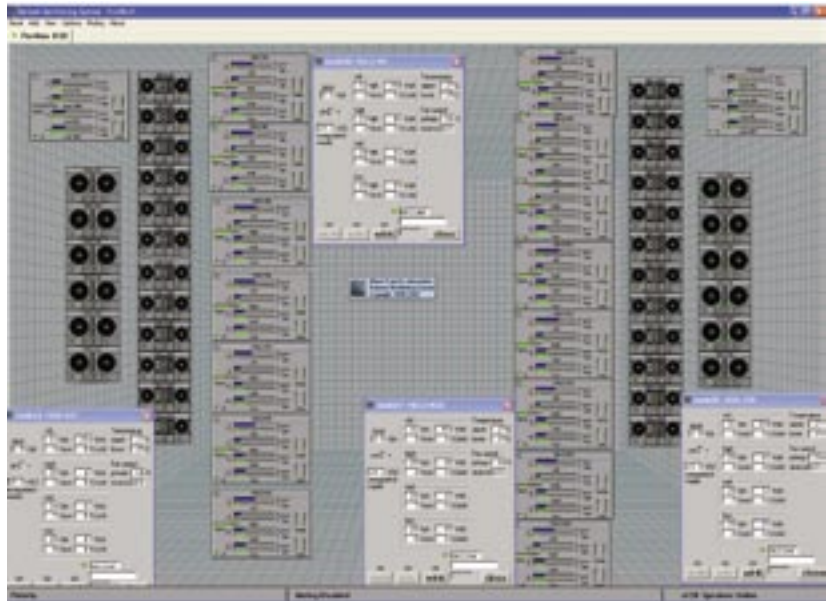
Figure 4.4: Sample RMS display panel showing MILO, MILO 120 and M3D-Sub loudspeakers.
