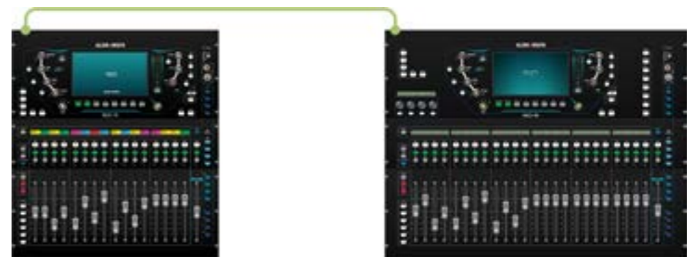
SQ + SQ 96kHz connection using gigaACE Send and receive all assignable I/O
